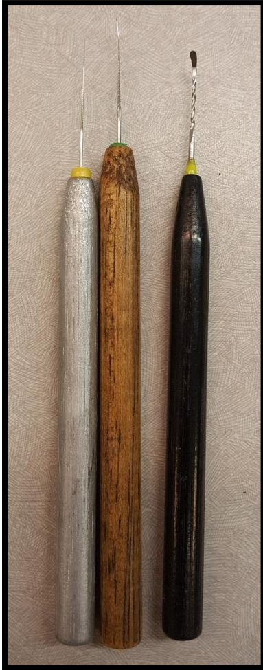
Figure 2. Microscopy tools; from left to right: 1) probe or single barbed tool; 2) bent probe; 3) minute spatula
